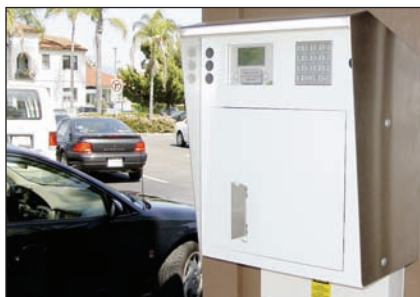
The automated Santa Barbara County Key-Manager Motor Pool Dispatch System at the Santa Barbara city location.
